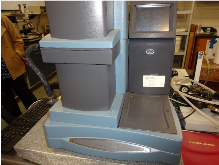
Dynamic Mechanical Analysis (Strength testing of polymer at Various temperatures)
